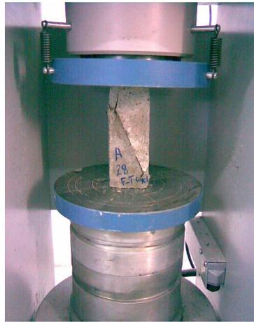
Figure 3. Slant shear test
