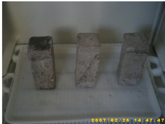
Figure 2. Samples of freeze and thaw test
