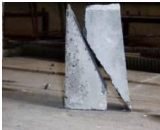
Figure 1. Concrete samples prepared based on BS 6319: Part 4
